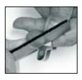
To make the upper register speak easily and with a bright tone, remove wood from the corners and tip. In doing this it is advisable to insert a plaque into the tip of the reed to prevent breakage. This operation is far safer if the reed is wet.
