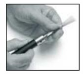
the inside of the reed. After it cools, be sure the throat is not obstructed with wax. A small rat-tail file will easily clean the throat. These operations should be done when the reed is dry.
