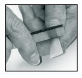
Most reeds are heavy and must have excess wood removed in the right places. If the lower tones do not speak easily and if the reed tires the lips, this is usually a sign that the wire end of the lay is heavy. Wood should be scraped or filed from the wire half of the lay.
