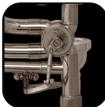
**Mechanical Style Trigger Linkage**
